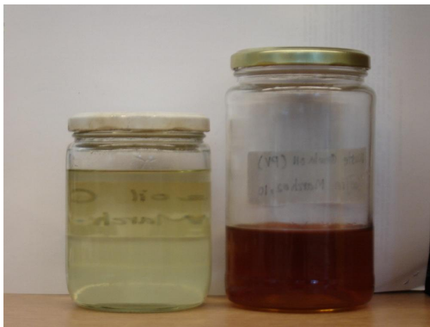
Figure 4.1. Fresh canola oil (left) and waste canola oil (right) from UBC Place Vanier residence
