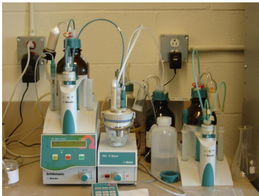
Figure 4.3. Karl Fisher volumetric titration apparatus for measurement of water content
